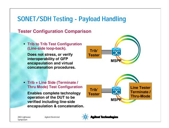
This first slide in this section highlights a simple, but important point. With regard to a dat over SONET/SDH MSPP equipment, GFP and virtual concatenation are line-side technologies. Therefore, to fully verify DUT compliance to the appropriate standards requires both tester stimulation and analysis of the line side. A test configuration involving only a client-side tester and line-side loopbacks will not achieve these required compliance checks.
