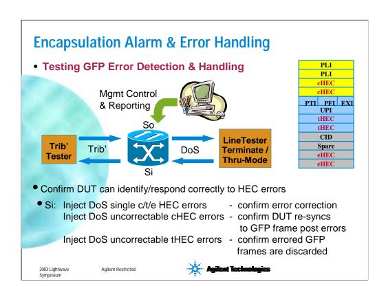
More complicated is the GFP error detection and correction test challenge shown on this slide. Again, as explained earlier, there are 3 categories of header error control - cHEC, tHEC and eHEC. This error control functionality can detect and correct single errors, but where there are more errors, the response of the DUT varies depending on the type of error.
