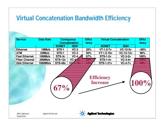
This table shows the improvements in bandwidth efficiency that can be made by using virtual concatenation instead of contiguous concatenation.
