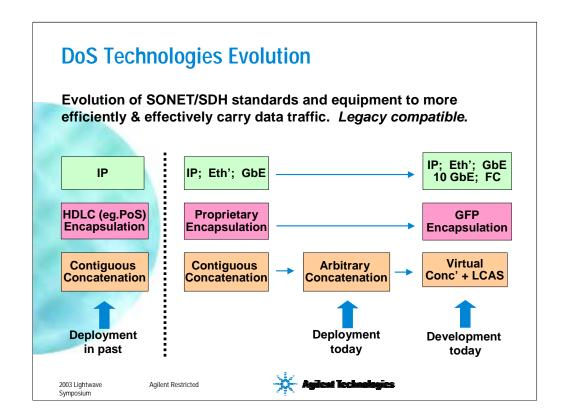
Against the backdrop of the simple technology layer model introduced in the last slide, this slide summarizes the data over SONET/SDH technology evolution. And I stress again - this is a LEGACY COMPATIBLE network evolution, not a NEW network revolution. Remember that all important cost driver.
