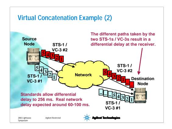
The two STS-1s / VC-3s in our virtual concatenated signal have taken different routes through the network and you will see that, at the destination node, frame 1 of STS-1 / VC-3 number 1 arrives 2 frames sooner than frame 1 of STS-1 / VC-3 number 2.
