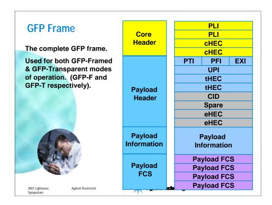
The basic structure of GFP frame comprises of a core header, followed by a payload header, payload information field and finally the payload FCS. The core header comprises of a **PLI or Payload Length Indicator field** which is guarded by a **Core Header Error Check or cHEC** which is a single bit error correction and multibit error detection techique.
