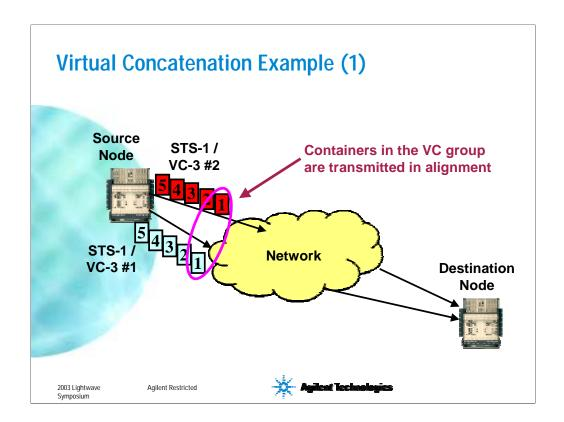
The pale blue boxes represent the SONET frames carrying the containers for STS-1 number 1 while the red boxes represent the SONET frames carrying the containers for STS-1 number 2.
