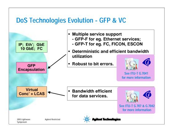
So what makes GFP the hot data over SONET/SDH encapsulation technology of today. Well, as this slide highlights, GFP suffers none of the drawbacks of the previously discussed encapsulation technique. In particular, GFP has been designed to support a variety of data service clients - a major benefit given that in the datacom world, one size certainly does not fit all! We will see how GFP achieves this flexibility later on in the seminar.
