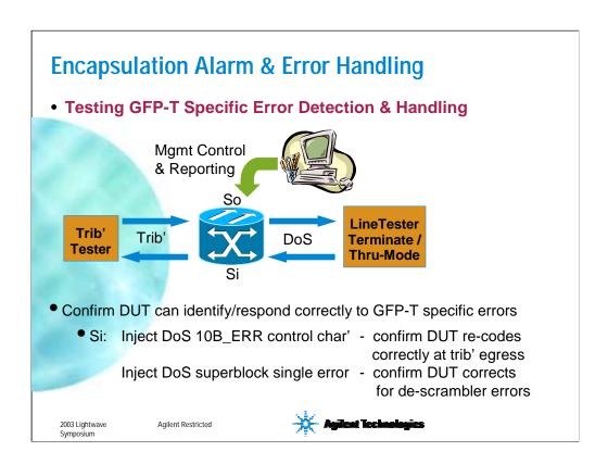
This slide highlights some test challenges specifically associated with the GFP-Transparent mode. GFP-T has some additional error conditions beyond the common conditions covered in the last slide. The specific examples shown here are:
