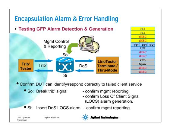
Consider first the verification of the GFP data encapsulation. As explained earlier, one of the major advantages of GFP over previous encapsulation techniques is it's robustness. Accordingly there are a number of error and alarm features which require verification. In particular, this slide highlights the testing of the GFP Loss of Client Signal alarm, which is fairly straightforward.
