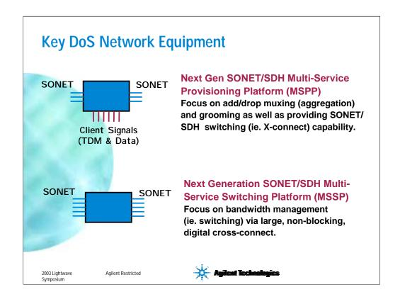
This slide outlines the two new equipment types dominating data over SONET/SDH networks. As their names imply, a key objective here is the support for multiple (ie varying) client service types. The MSPP sits at the edge of the network and is the ingress and egress point for the client signals onto the SONET/SDH network. An MSPP can typically aggregate and groom client signals of varying types, as well as digitally switching (ie X-connecting) SONET/SDH signals.
